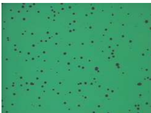
Figure 3. Example of the formation of black spots in electroluminescence of a OLED as a result of storing the device at ambient conditions for a few days. The area of the picture is approximately 3 mm 2 .
