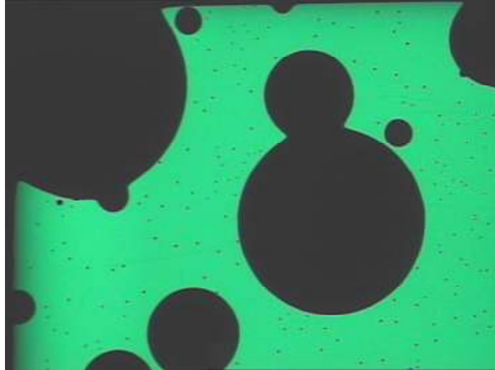
Figure 8. Electroluminescence from an OLED device ( 2 \times 1.5 mm 2 ) encapsulated with a SiN-layer after exposure to the ambient atmosphere for one year. The large black spots correspond to pinholes that are not covered by the SiN layer. The tiny ones correspond to pinholes that are covered by SiN. The growth of the tiny spots is limited by the WVTR of the SiN layer ( 10^{-5} g/m 2 /day)
